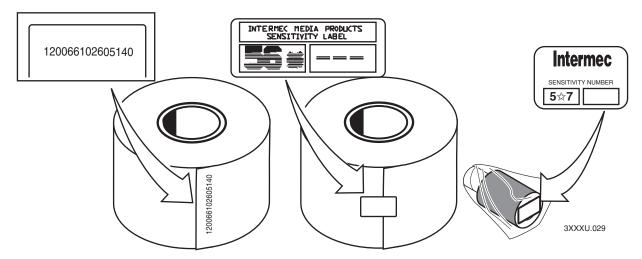
**Media sensitivity number:** This illustration shows you where to find the media sensitivity number. Note that some ribbon rolls have the media sensitivity number printed inside of the core.
